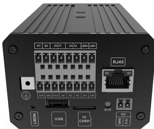
2-3 Schematic diagram of camera wiring interface.
