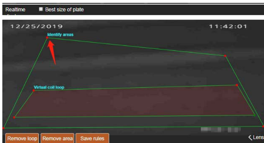
3-8 Virtual coil and recognition area
